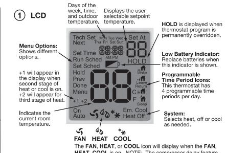
HEAT, COOL is on. NOTE: The compressor delay feature is active if these icons are flashing. The compressor will not turn on until the 5 minute delay has elapsed. These may also flash for staging delay or floor sensor override.
