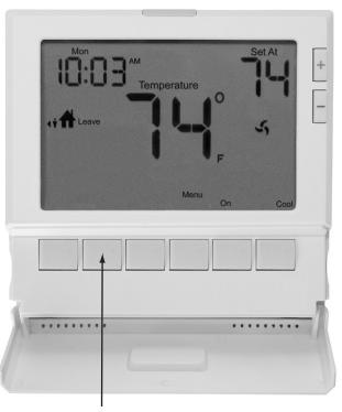
Hold down for 3 seconds, to reset filter reminder.
